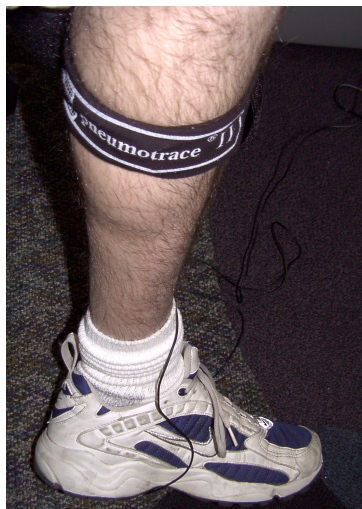
Figure 6. Attachment of the respiratory belt transducer to the calf for leg volume measurement.
